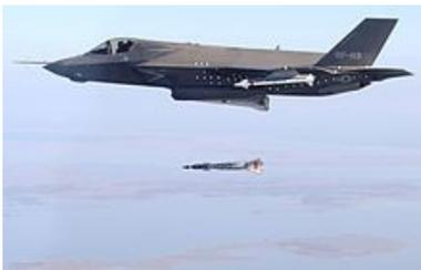
The 500-pound GBU-12 general purpose bomb carried a nose-mounted laser seeker and flight guidance fins for precision strike was released at 25,000 feet and the bomb fell for 35 seconds before hitting a tank on the Edwards Air Force Base test range. The aircraft used its Electro-Optical Targeting System (EOTS) to enable the pilot to identify, track, designate and accurately deliver the GBU-12 on target.
